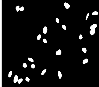
Figure 39: Segmentation mask with fused objects
