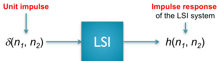
Figure 24: Impulse response of a system
